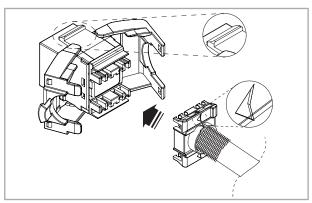
4. Check that the wired cap is in the correct orientation and cover it with both jaws.
