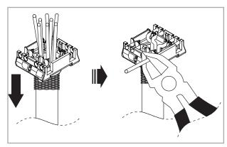
3. Weave the cable end through the cap. Seat each color coded wire into the matching cap position and trim excess wire.
