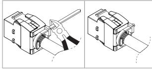
5. Thread the supplied cable tie through the wired cap, then tighten around the braided shield. Trim the cable tie.
