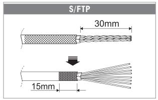
1. Remove about 3cm of the cable sheath. Keep about 15mm of the cable braid (foil).
