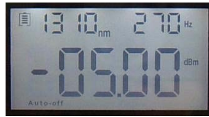
Laser on (output wavelength 1310nm; rated output power-5.00dBm;270Hz frequency)
