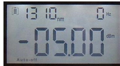
Laser on (output wavelength 1310nm; rated output power-5.00dBm; 0Hz: no frequency set.)
