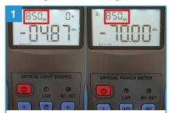
Turn on the light source (OLS) and power meter (OPM) and set each device to the same wavelength by pressing the  $\lambda$  button.
