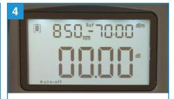
With the OLS and OPM connected, quickly press the **REF** button (OPM) to zero the calibration. The dBm value will move to the top-right corner, replaced by "00.00 dB" in the main LCD area.
