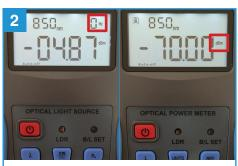
On the OLS, press the CW button until  ${\bf 0}$  Hz is displayed. \*Dashed lines indicate laser is off. Press  ${\bf \lambda}$  button to activate laser.
