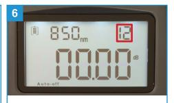
To save test results in the OPM, press the **SAVE** button to see the reference number, then press **SAVE** again to store the record. 1000 records may be stored.
