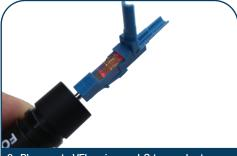
Place onto VFL using an LC type adapter.
