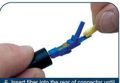
Insert fiber into the rear of connector until a slight "bow" is created and the light emitting from connector window dims and/or extinguishes.
