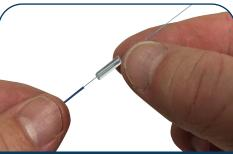
2. Slide included 900µm build tube section onto fan tubing.\*\*
