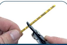
2. Using strippers remove approximately 50mm / 2" of cable jacket.
