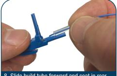
Slide build tube forward and seat in rear of connector, ensure fiber is straight, close hinge. Slide boot forward and tighten until secure.
