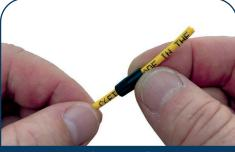
Unscrew boot from rear of connector and slide onto cable jacket. For 2.0mm slide included build tube onto cable jacket.\*\*
