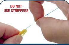
Pull Kevlar yarns back to locate SSF<sup>™</sup> fiber. Use only finger tips/nails to gently remove "Soft Peel" 250µm coating to within 12mm/1/2" of cable jacket. ¹
