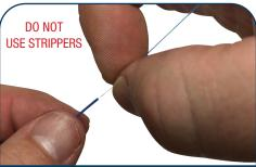
Use only finger tips/nails to gently remove "Soft Peel" 250μm coating completely to fan tubing.
