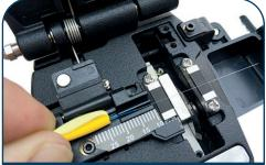
Cleave fiber measuring from cable jacket.
