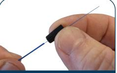
Ensure a minimum of 50mm of fiber exits the fan tubing. Unscrew boot from rear of connector and slide onto fan tubing.
