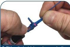
Slide activator tab towards connector tip. Remove from VFL, Install dust cap.
