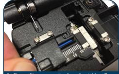
Cleave fiber measuring from fan tubing. For SSF™ LC = 12mm.<sup>2</sup> Fiber must extend across both black pads to successfully cleave.
