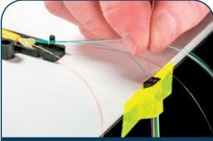
Ensure the fibers are not twisted around each other as they enter the block as this may cause attenuation from micro-bends at the point where they enter the block.
