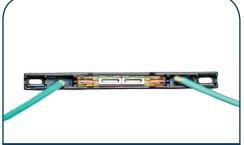
15. Carefully remove splice and fiber cable from tool and place into splice assembly.
