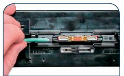
Insert cleaved fiber into the left opening of splice by placing in v-groove at a slight angle. Slide forward until jacket touches side of black splice holder.
