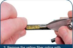
3. Remove the yellow fiber splice with fingers or sharp edge. Avoid touching fiber opening. Place in splice installation tool.
