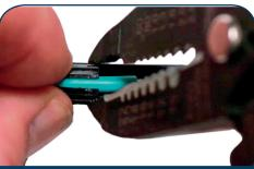
16. Place jacket sleeve ring on cable, ensuring it is over sleeve windows and fiber is straight. Squeeze ring carefully with pliers to inset into place. Repeat for left cable.
