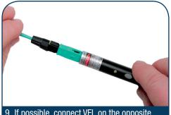
9. If possible, connect VFL on the opposite end of one of the fibers being spliced for verification purposes.
