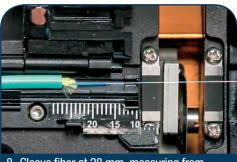
8. Cleave fiber at 28 mm, measuring from jacket.
