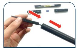
OPTIONAL: For outdoor application, insert heat shrink tubing on end of cable to be spliced.
