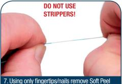
Using only fingertips/nails remove Soft Peel 250 μm coating completely from the fiber to within approximately 12 mm or ½" of the cable jacket. Repeat process for other cable.
