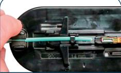
Insert cable under slide arm and place into foam holders so cable lays straight. Repeat the previous cleaving process for the right cable fiber leg to be joined.
