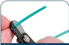
Using the appropriately sized opening on strippers for cable being spliced, remove approximately 50 mm/2" of the cable jacket. If needed, install build-up tube.
