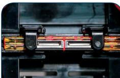
14. Maintain forward pressure and loss of light while pushing each of the two slide arms towards the center. Slide the metal tabs until they touch to lock in the fibers.
