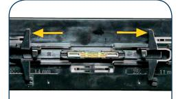
4. Slide each of the two assembly activator slides away from the center of the tool.
