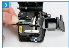
Open the cleaver. Align the end of the jacket at the 24mm mark, close the top, then quickly push the button(•) to complete the cut.
