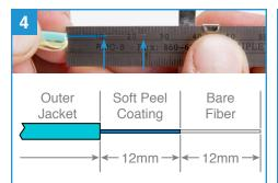
Measure the fiber. A properly cleaved end measures 24mm from the jacket to the tip of the fiber (12mm of coating and 12mm of bare fiber).
