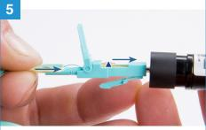
Push the fiber into the connector opening until it bends slightly and the VFL light dims, then push the activator slide tab (A) toward the VFL to lock the fiber in place.
