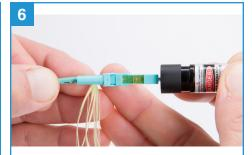
Fold the Kevlar strands to one side and hold the clamshell cover closed. Remove the connector from the VFL and replace the dust cap.
