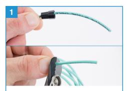
Slide the threaded boot on the end of the cable, then cut the fiber jacket back 2" using the strippers.
