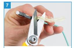
Thread the coonector boot on enough to catch the Kevlar strands, then trim the strands and thread the boot on the rest of the way.
