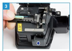
Open the cleaver. Align the end of the jacket at the 28mm mark, close the top, then quickly push the button(•) to complete the cut.
