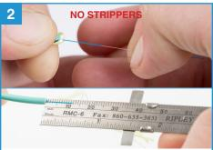
Using your fingernails, scrape the soft peel coating, leaving 12mm of coating between the jacket and the exposed fiber. \*Important: Do not use strippers to remove the soft peel coating.
