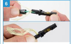
Remove the connector from the VFL and replace the dust cap. Fold the Kevlar strands to one side and close the clamshell.
